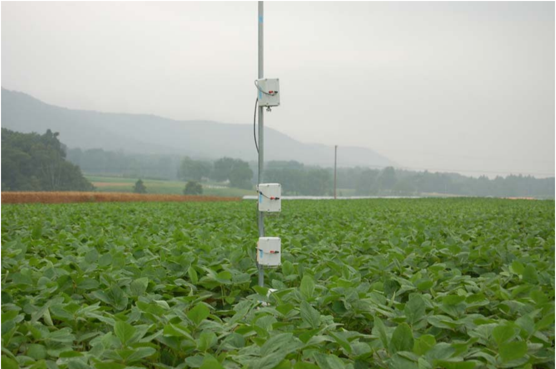
Fig. 2.1: The location of the rotorods on the tower relative to the height of the canopy h . Concentration profiles can be estimated by collecting spores or particles with rotorods located at each height on a tower.
