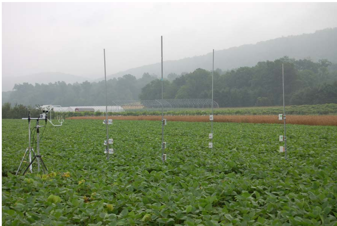
Fig. 2.2: Location of meteorological and collection instruments during a particle escape trial in Rock Springs, PA. A similar design was used for each of the three experiments.
