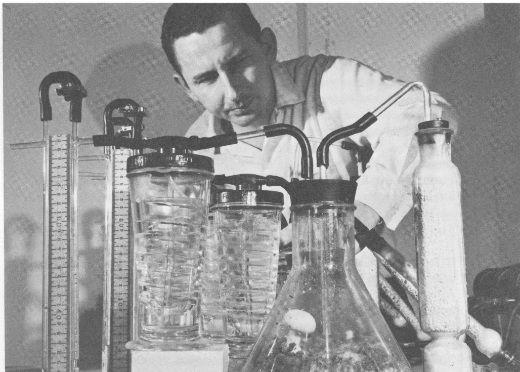
Apparatus used to study gas relationships of mushroom spawn
